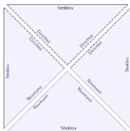
FIGURE 2. Decomposition of the Steklov problem on a square into four mixed problems on a triangle.
