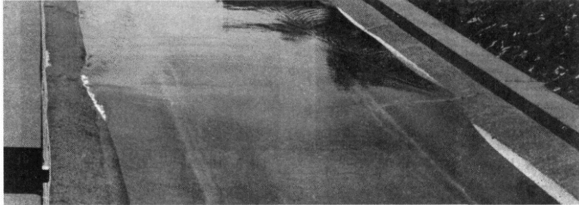
Fig. 8. Undular bore at Froude ~ 1.04.
