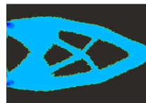
Figure - Optimized shape for a vertical load
