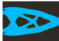
Figure - Optimized shape for an uncertain load
